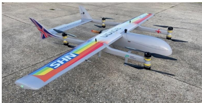
Figure 4. Skylift Mugin V50 VTOL-fixed-wing drone used in Trial 2
