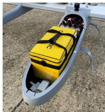
Figure 6. Aseptic medicine carrier loaded into the drone. Same dimensions as the medium carrier (left). Loaded weight ~5kg.
