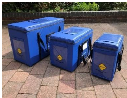
Figure 5. Empty medical carriers carried in Trial 1. Approx. dimensions of the medium (middle) carrier = 46 cm × 26 cm × 31 cm. Total loaded weight ~10kg.
