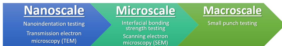
Figure 1. The scope of the experimental multiscale framework of microstructural and mechanical characterization of copper – silicon carbide composites.
