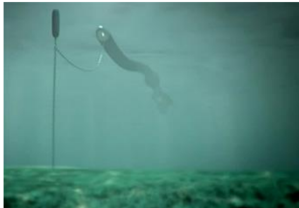
Figure 1.1 An imaginary impression of Anaconda wave energy convertor (provided by Checkmate SeaEnergy Ltd [48])
