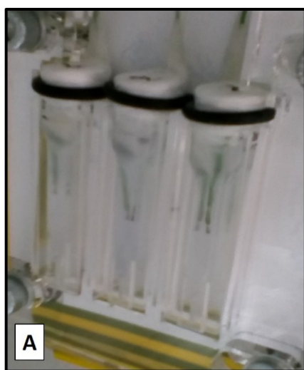
Set-up A , 3 x 1.5 mL samples in ZEN0040 micro-cuvettes with dimensions – 46 mm H x 4 mm W x 10 mm D
