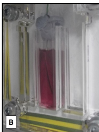
Set-up B , 1 x 3 mL sample in cuvette with internal dimensions – 45 mm H x 10 mm W x 10 mm D
