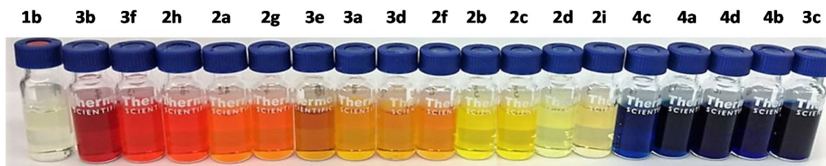
Figure 6. Photograph of 1 mM solutions of the starting material 1b (left) and cross-coupled products 2a–4d in chloroform under white light.
