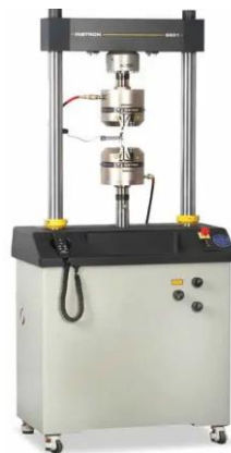
Figure 3-16 Instron servohydraulic testing machine from Instron website
