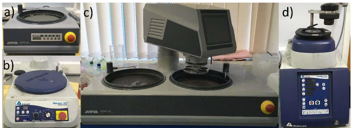
Figure 3-8 Pictures of the turntables used during metallographic preparation. a) ATM Saphir 350 grinding machine, b) Buehler MetaServ 250 polishing wheel, c) ATM Saphir 560 automatic polisher, d) Buehler SimplyMet XPS1 mounting press. Pictures from [58]
