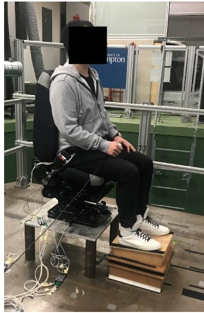
Figure 5.3 One subject seated in the suspension seat with upright backrest
