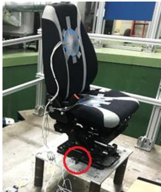
Figure 5.1 The suspension seat, the SIT-pads (blue) and single-axial accelerometers (circled) used in this study
