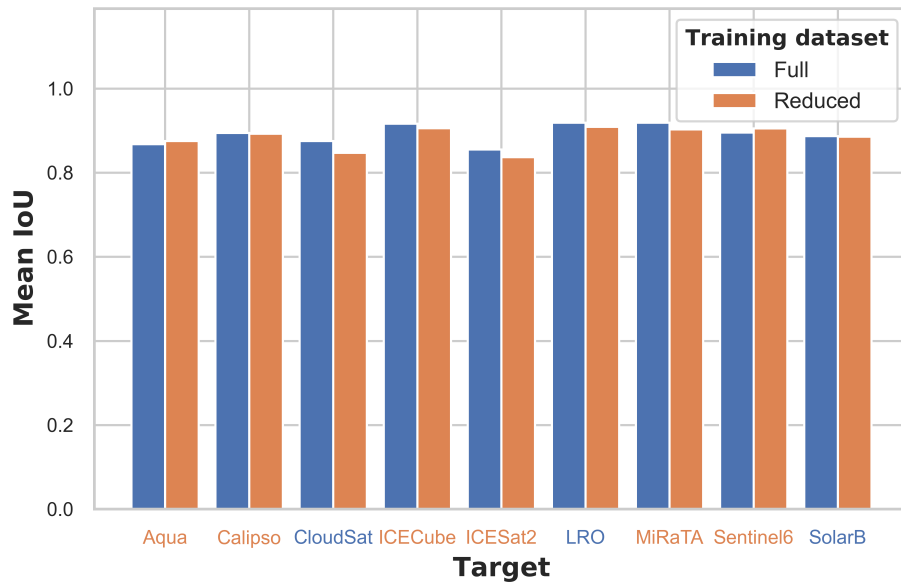
FIGURE 3.5: Difference in mean IoU values between targets which have been seen during training and those which have not. Targets with names in blue are in the full dataset only; those with names in orange are in both.
