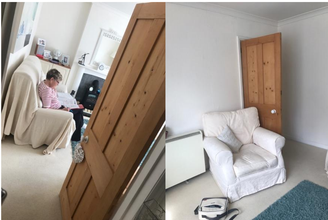
figure 4.19 knob door handle is not easy to grab, and the open direction of the door make room feel smaller
