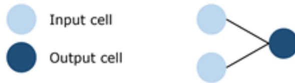
Figure 3: A single-layer perceptron
