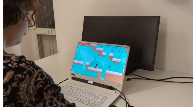
Figure 2: Experimental setup: A participant performing the experiment on a laptop computer equipped with an eye tracker.
