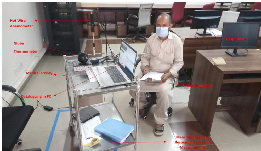
Fig 02. Field Assessment Typical Setup with Instrumentation and Respondent
