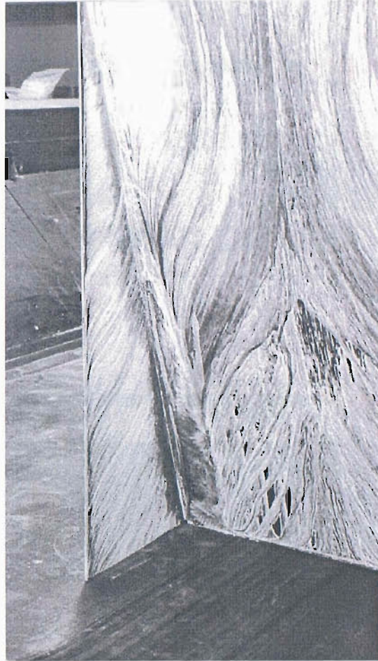
Figure 33: Type A surface flow at inner side-plate, h_r/d=0.382 . Flow direction from top to bottom.
