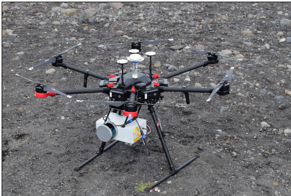
FIGURE 32 Example of a customised UAV system for use in geomorphological research. In this instance, the UAV is a DJI M600 which has been equipped with a velodyne VLP-16 laser scanner for surface height measurements (carried under the UAV) as well an on-board IMU to allow for much greater positional accuracy than given by traditional GPS receivers.
