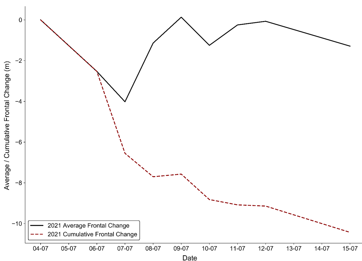
FIGURE 61 Average and cumulative frontal change for July 2021, calculated using the rectilinear box method.
