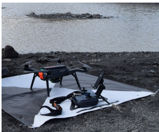
FIGURE 39 The 3DR Solo quadcopter used to undertake the UAV surveys in July and September 2019.
