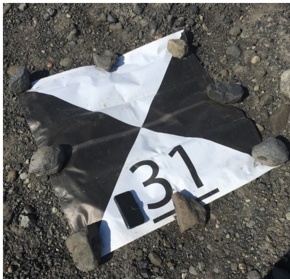
FIGURE 41 Example of one of the 1x1 m GCPs placed in the vicinity of Fjallsjökull to georeference the glacier models to real-world coordinates.
