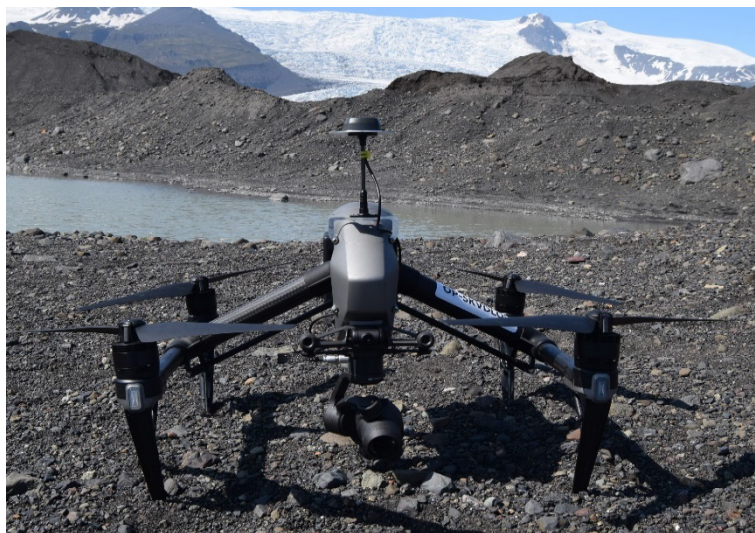
FIGURE 43 The DJI Inspire 2 used to undertake the UAV surveys in July 2021. Note the GNSS antennae fixed to the top of the UAV body to allow for direct georeferencing capabilities.
