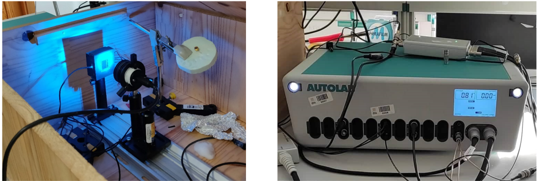
FIGURE 3.2: Example of the apparatus required for an impedance spectroscopy measurement. Left image shows a cell under illumination with wire connections to an ‘Autolab/PG-STAT302N’ potentiostat (right) which applies the voltage perturbation and measures the current response. A frequency response analyser module is used to extract the phase and amplitude from the current response.
