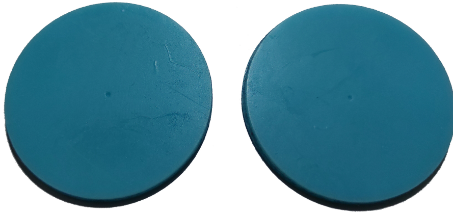
(a) Void sides of the printed cell showing the central void and a much flatter surface
