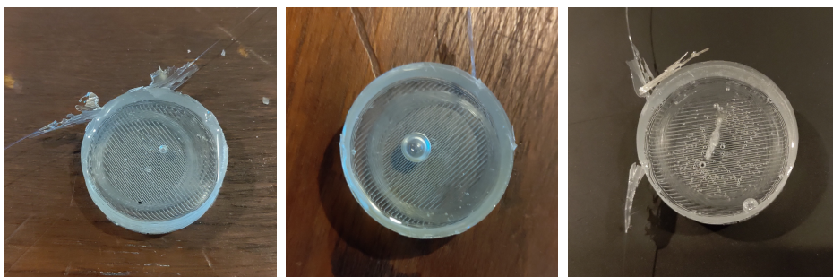
(a) Small void (0.5 mm) (b) Large void (2.5 mm) (c) Failed cell with gouge instead of void
