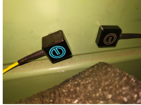
(b) Picture of the two sensor heads with differing cavity resonances: the larger left sensor at 50 kHz, and the smaller sensor on the right at 200 kHz
