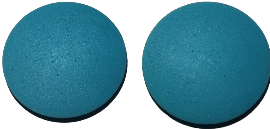
(b) Flat sides of the printed cell showing voids from trapped air bubbles
