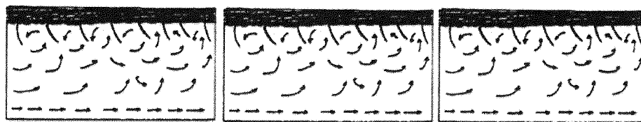
FIGURE 2.10: Observation of the flow between different surface smoothness (Rushall et al., 1994). From top to bottom: skin with hair, smooth skin but with hydrophobic surface, smooth granulated surface (i.e. shaved skin).
