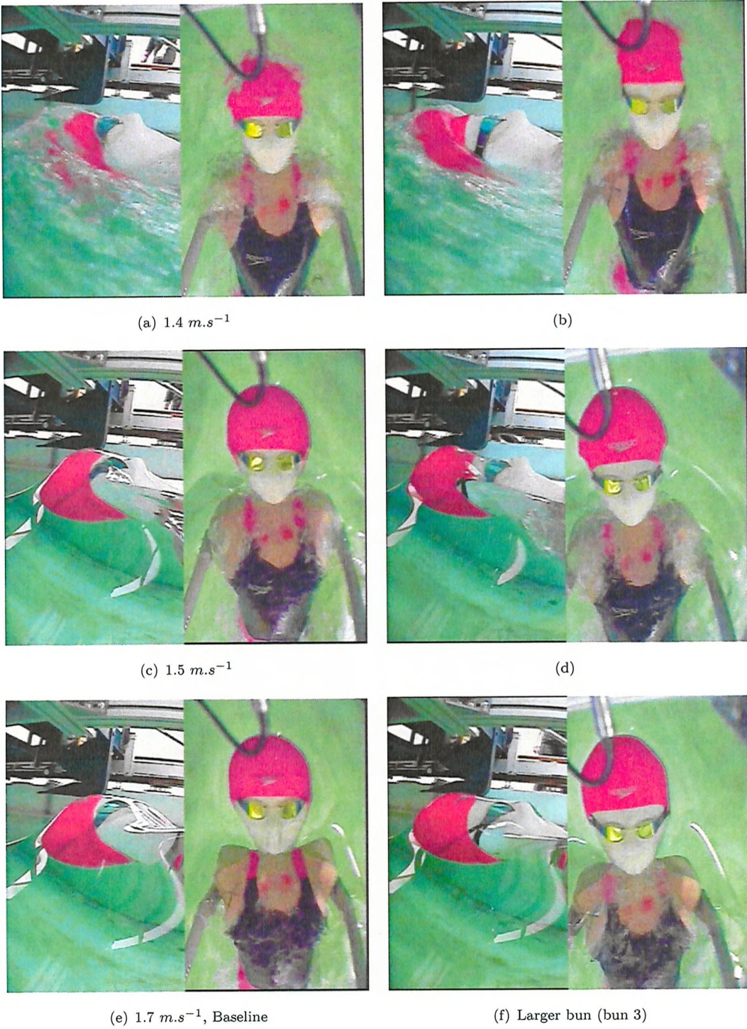
FIGURE 8.24: Flow visualisation of baseline versus large bun (bun 3) on the mannequin on back.
