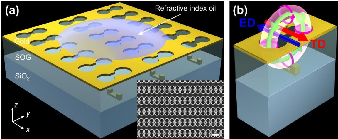
93 **Fig. 1** (a) Schematic diagram of the proposed anapole metamaterial array for refractive index sensing.
