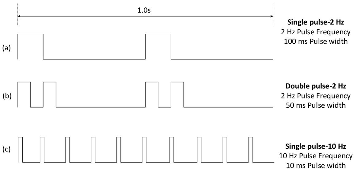
Figure 4.5. Three PDC waveforms: (a) single pulse- 2 Hz, (b) double pulse- 2 Hz, and (c) single pulse- 10 Hz waveforms used to investigate European eel (silver-phase) response to electric fields under static water conditions (Experiment 1).
