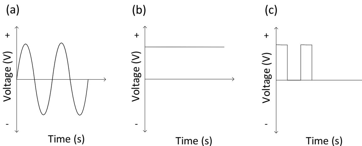
Figure 2.2. Diagram of examples of three types of electric current: (a) alternating current (AC), (b) direct current (DC) and (c) pulsed direct current (PDC).
