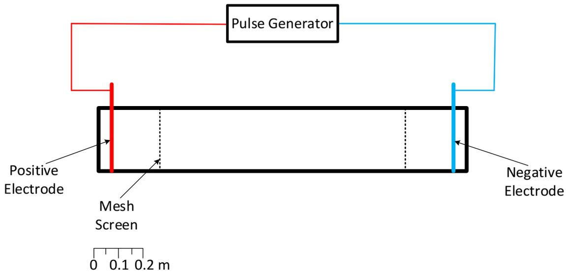
Figure 4.1. Section of rectangular tank used to quantify thresholds of eel response to electric fields under static water conditions. Two aluminium electrodes were placed at either end of the tank and connected to a voltage pulse generator used to create the electric field.
