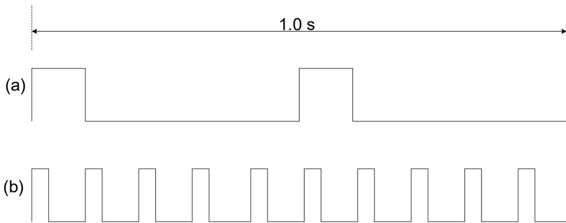
Figure 5.2. PDC frequencies (a: 2 Hz; b: 10 Hz) used to investigate juvenile eel response to electric fields in flowing water.
