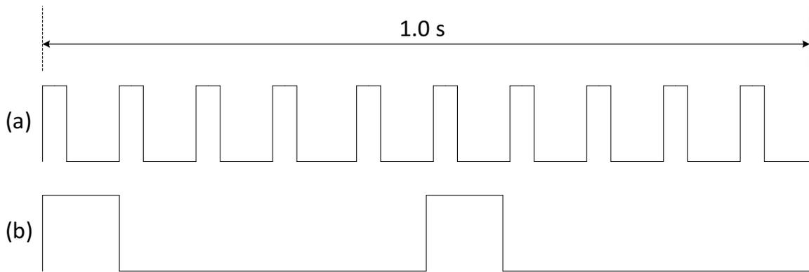
Figure 6.2. PDC frequencies: (a: 10 Hz; b: 2 Hz) used to investigate European eel response to two-choice test electric field. The 10 Hz frequency was used for yellow-phase eel (experiment 1) and both frequencies were tested in silver-phase eel trials (experiment 2).
