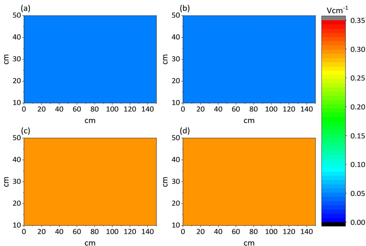
Figure 4.2. Electric field ( $\text{Vcm}^{-1}$ ) generated in the static water tank. (a) and (b) represent field strengths obtained with a pulse generator output of 7 V. (c) and (d) represent field strengths obtained with a pulse generator output of 42 V. (a) and (c) were measured at 5 cm depth and (b) and (d) at 10 cm depth from the water surface. Electric field strength was uniform across the tank and proportional to input voltage.
