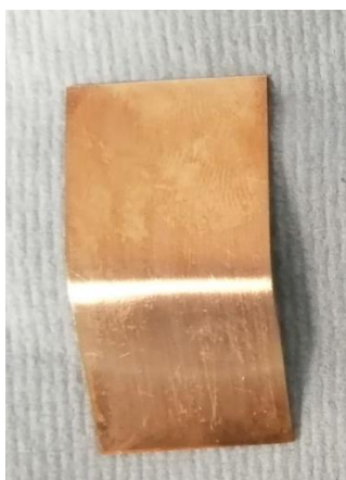
Figure 95 - Result of the silver corrosion test obtained from the oil sample B after being subjected to our reclamation process with polymer C.
