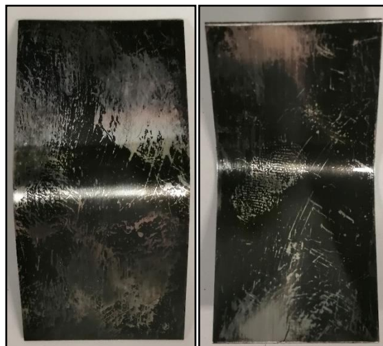
Figure 63 - Corrosion test result of the oil sample spiked with 1 ppm of S_8 subjected to the standard corrosion test (DIN 51353). The silver strip (showing both sides) presents black colouration (silver sulfide), which indicates that the oil is corrosive.
