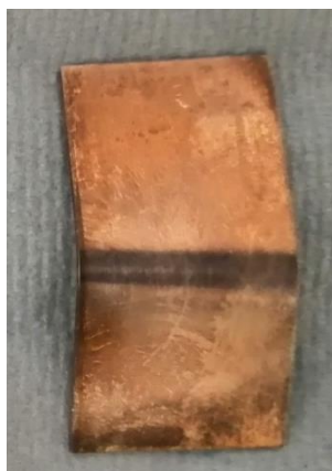
Figure 96 - Result of the silver corrosion test obtained from the oil sample B after being subjected to our reclamation process with polymer D.
