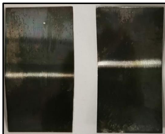
Figure 59 - Corrosion test result of the ex-service mineral oil sample B subjected to the standard corrosion test (DIN 51353). The presence of the black colouration (silver sulfide) indicates that the oil is corrosive.
