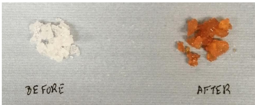
Figure 94 – Change in colour of the polymer B due to reclamation process of the oil sample B.
