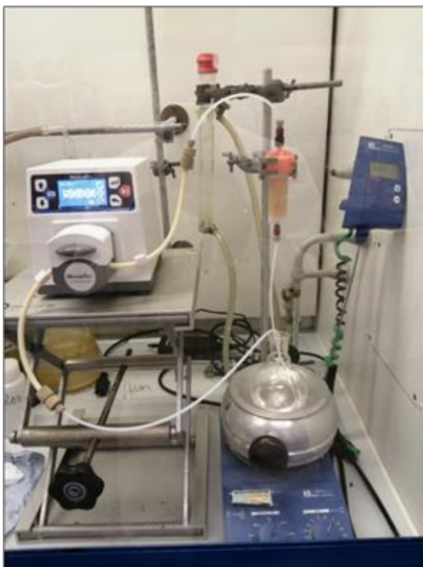
Figure 89 - Optimised laboratory reclamation rig set-up used for the selective removal of elemental sulfur from mineral oil.
