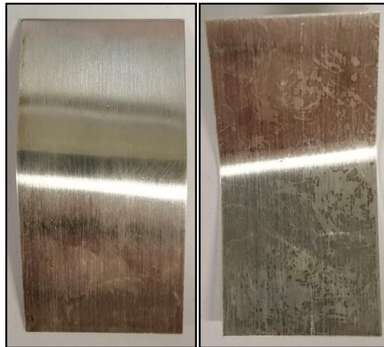
Figure 62 – Silver strip (showing both sides) used as reference for the standard DIN 51353 corrosion tests.
