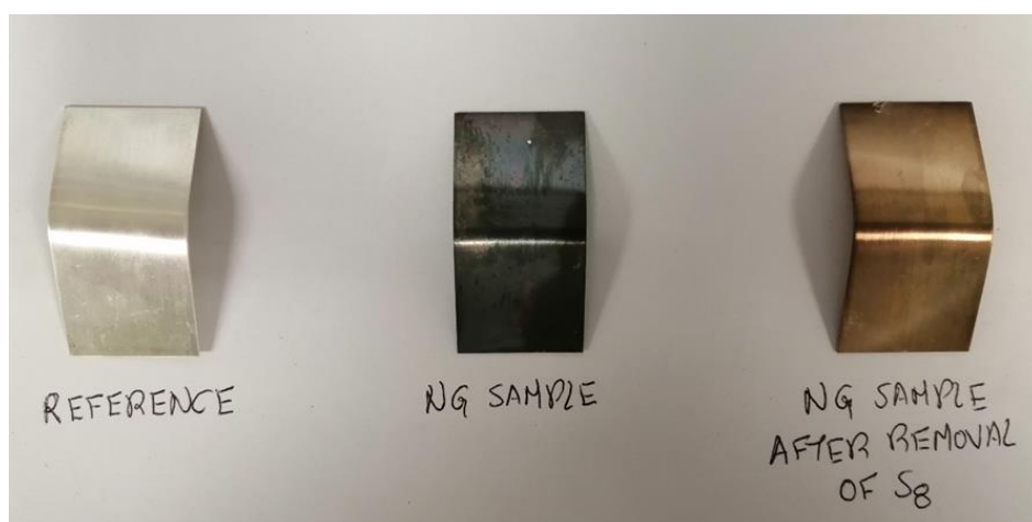
Figure 92 - Result of the silver corrosion test obtained from the oil sample B after being subjected to our reclamation process with polymer A. * Yellow colouration is due to the thermal stress.
