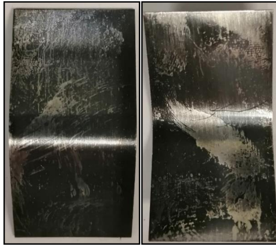
Figure 64 - Corrosion test result of the oil sample spiked with 2 ppm of S_8 subjected to the standard corrosion test (DIN 51353). The silver strip (showing both sides) presents black colouration (silver sulfide), which indicates that the oil is corrosive.
