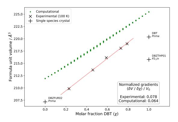
**Figure 8.** Plots of the formula unit volume of *Pnma* mixed crystals of DBT and DBF as a function of  $\chi_{DBT}$ . Experimental data points (×) were obtained by single-crystal X-ray diffraction at 100 K (Table 4). Computational results (green dots) exhibit a similar volume increase in simulated *Pnma* mixed crystals. The plot also includes reported values of formula unit volume (+) for  $P2_1/n$  crystals of pure DBT at 100 K and for *Pnma* crystals of pure DBF at 169 K.<sup>32,47</sup>
