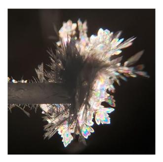
**Figure 10.** Sublimed crystals of pure DBT imaged by optical microscopy under polarized light. The thin plates correspond to the metastable Pnma polymorph and the needles to the previously reported  $P2_1/n$  form.
