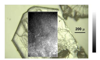
**Figure 5.** Optical micrograph showing a mixed *Pnma* crystal grown from a solution in MeOH containing an initial DBT:DBF ratio of 2:3, with an overlaid compositional map of a rectangular part of the crystal obtained by Raman microscopy. Local composition was determined by measuring the relative intensities of characteristic Raman bands ( $v_{701}$  for DBT and  $v_{730}$  for DBF). The scale ranges from black to white as the local value of  $\chi_{DBT}$  increases from 0.33 to 0.50.
