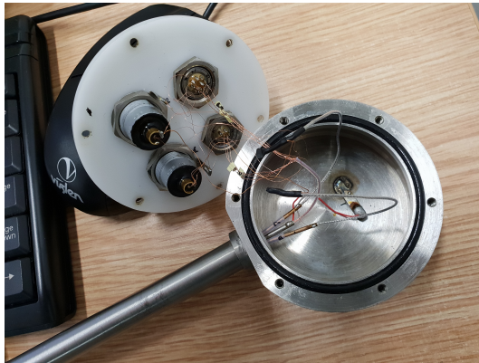
(a) Old Cryogenic sample insert with low signal-noise wiring.
