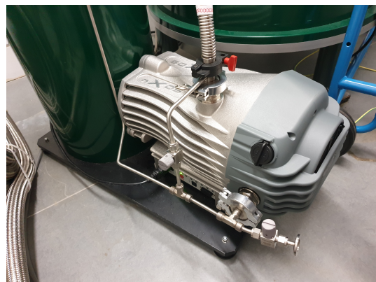
(d) New scroll pump fitted for continuous cryostat operation.
