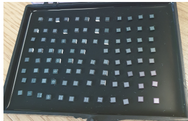
(c) Post laser cut sub-chips
