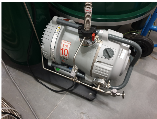
(c) Failing scroll pump with worn out bearings.
