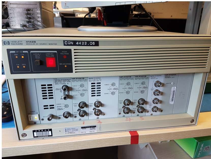
FIGURE A.1: HP4142 measurement system after installation of new SMUs.
