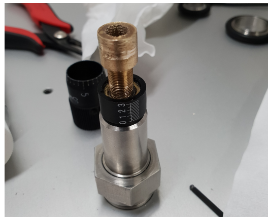
(e) Replacement of needle valve in order to reach stable temperatures below 4.2 K.
