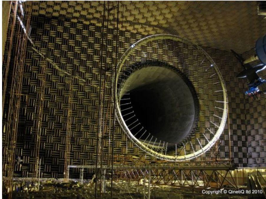
FIGURE 6.9: View of the NTF showing jet nozzles, exhaust gas collector and microphone arrays
