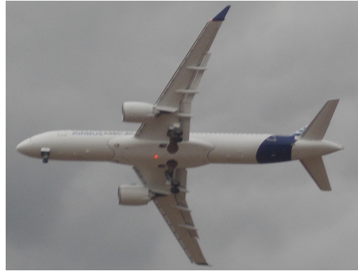
FIGURE 5.35: View of the underside of an Airbus A220, displaying the unswept and swept portions of the wing trailing edge
