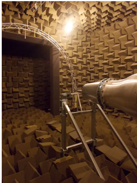
FIGURE 3.1: Doak Laboratory with jet and flight stream. Also shown is the aerofoil support structure and, at the top of the figure, the flyover microphone array used to measure far-field jet noise
