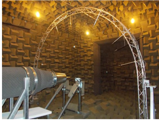
FIGURE 3.7: Azimuthal array positioned at a polar angle of 90^\circ to the jet nozzle exit
