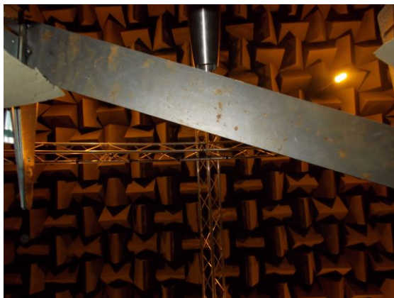
FIGURE 3.8: Swept plate with a chord of 2.5D and sweep angle of 20^\circ
