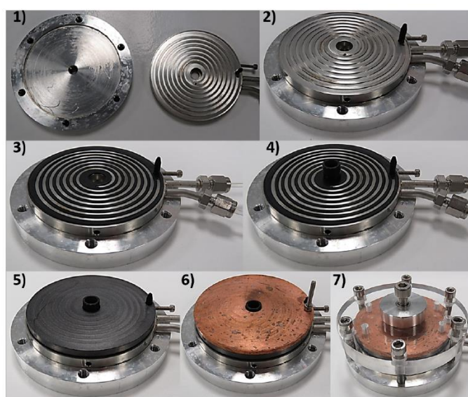
Figure 4. 3: how to assemble the cell.
