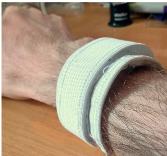
Figure 6.1: Image of the custom made mosaicOne_C haptic device. The device houses 4 306-10H 7-mm haptic motors, spaced equally around the wrist.
