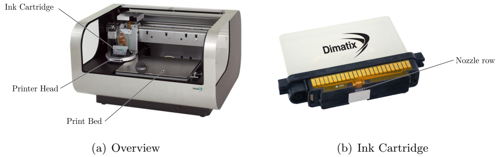
FIGURE 2.6: Dimatix Materials Printer DMP2831 [82]: (a) Overview ; (b) Ink Cartridge
