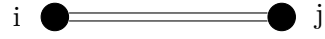
Figure 4.3.7: Z^2 operator between two nodes. For qubits Z^2 = \mathbb{I} this is the same as the two nodes being disconnected.
