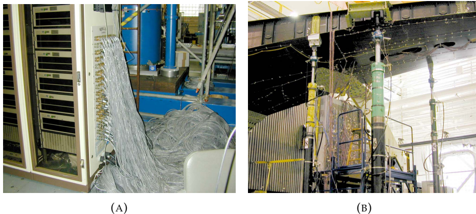
FIGURE 1.1: Photographs showing (a) the cabling required to connect 466 foil strain gauges to (b) the stitched/resin film infused graphite-epoxy wing box, a test article as part of an aircraft design process. Reproduced from [16].
