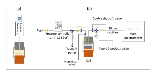
Figure 1. Schematic of the operando pressure cell (a) and the on-line electrochemical mass spectrometry (OEMS) setup (b).
