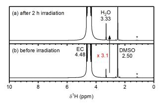
Figure 8. <sup>1</sup>H NMR spectra of an ethylene carbonate (EC) and Rose Bengal (100 μM) solution (a) after and (b) before 2 hours of irradiation at 525 nm to generate singlet oxygen (<sup>1</sup>O<sub>2</sub>). The chemical shifts of EC, H<sub>2</sub>O and DMSO are annotated in black. An enlarged spectrum is given in Figure S25. After generation of <sup>1</sup>O<sub>2</sub> in solution, the H<sub>2</sub>O signal increased 3.1 times.
