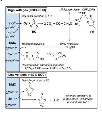
Figure 11. Overview of the electrolyte decomposition reactions that occur at the positive electrode at high potentials (state-of-charge, SOC >80%) and low potentials (SOC <80%). The formal oxidation states of the transition metal ions are indicated with superscripts (x, x' and x") and are illustrative.
