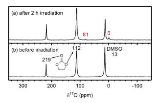
Figure 9.  $^{17}O$  NMR spectra of an ethylene carbonate (EC) and Rose Bengal 100  $\mu$ M) solution (a) after and (b) before 2 hours of irradiation at 525 nm to generate  $^{17}O$ -enriched singlet oxygen ( $^{1}O_{2}$ ). The chemical shifts of EC (219 and 212 ppm) and DMSO (13 ppm) are annotated in black. The chemical shifts in red correspond to the signals for water (0 ppm) and dissolved  $CO_{2}$  (tentatively, 81 ppm), the signals appearing after  $^{1}O_{2}$  production in solution.
