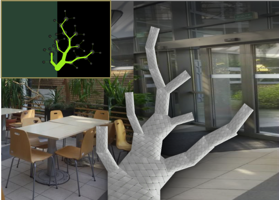
Figure 3: An example VMC structure in simulation (inset image) to guide the branching of braids and the number of filaments in each branch. This sketch shows a braided scaffold that is attracted and growing towards the space at the right side because it is infrequently occupied by furniture or people.
