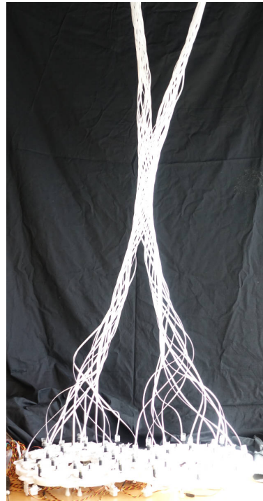
(c) Filament is connected to dispensers which are driven by the modules to create braided structures.
