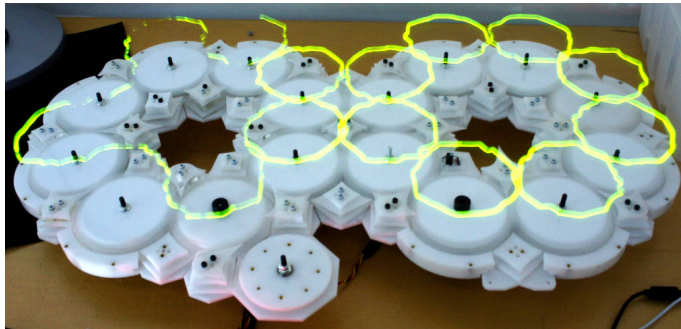
(b) 16 Modules assembled as two circles of each 8 modules. The circles are connected over two driver modules, and share one switch module.
