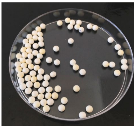
Figure 2.6. (Left) UiO-66@alg beads after heat treatment. 36 Reproduced with permission from Elsevier.
