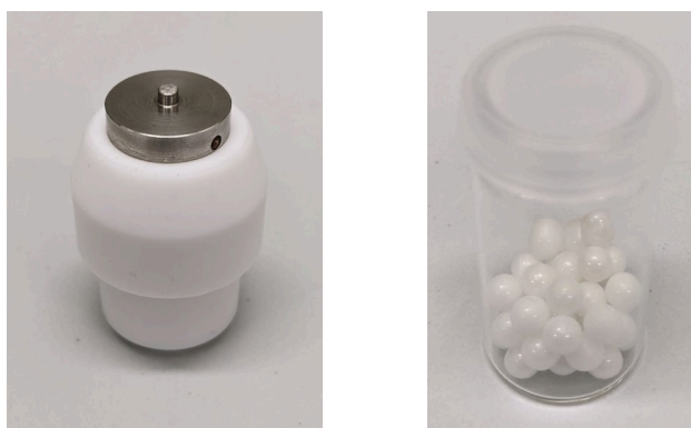
Figure 1.24. Teflon ball milling vessel and zirconia balls that are used in ball milling.
