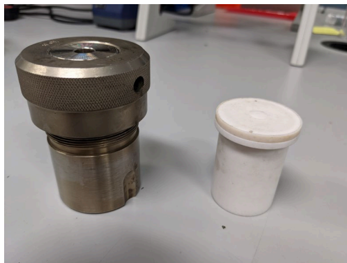
Figure 1.23. Steel autoclave reactor and Teflon liner that fits within the autoclave.
