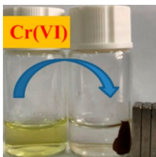
Figure 1.39. Chromate removal by a Cu MOF@ \text{Fe}_3\text{O}_4 composite and the easy separation of the material from solution with a magnet. 185 Copyright 2018 American Chemical Society.
