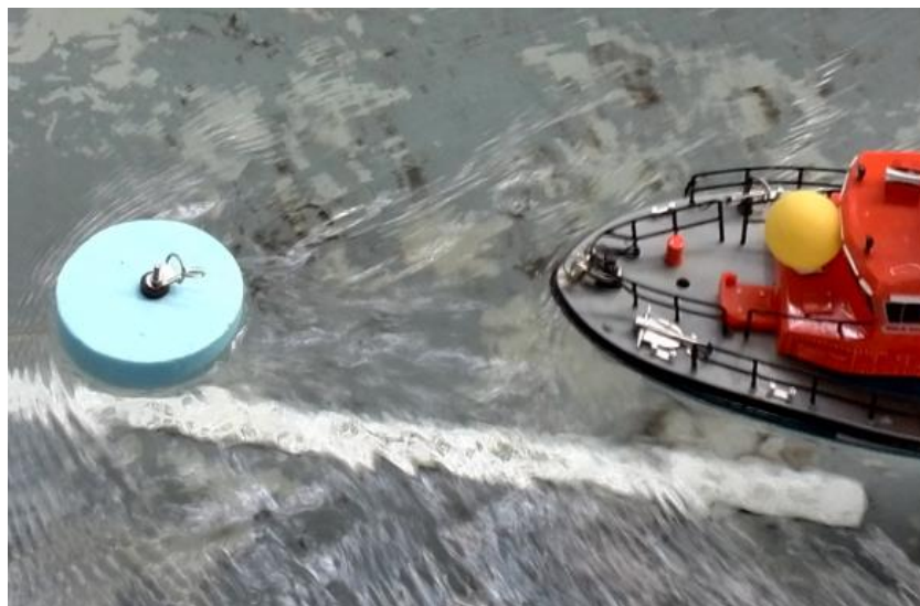
Fig. 15: Turbulent wake created by 1:20 scale buoy.
