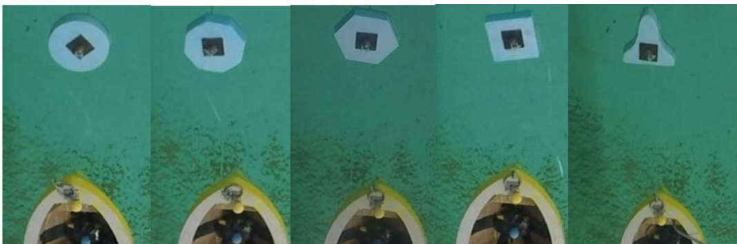
Figure 33: Five 1:10.67 scale buoy shapes tested in regular waves.
