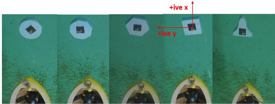
Fig. 2: 1:10.67 scale buoy shapes and 2D frame of reference.
