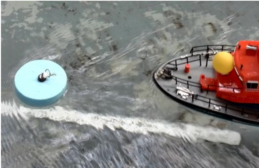
Figure 30: Turbulent wake created by 1:20 scale buoy.
