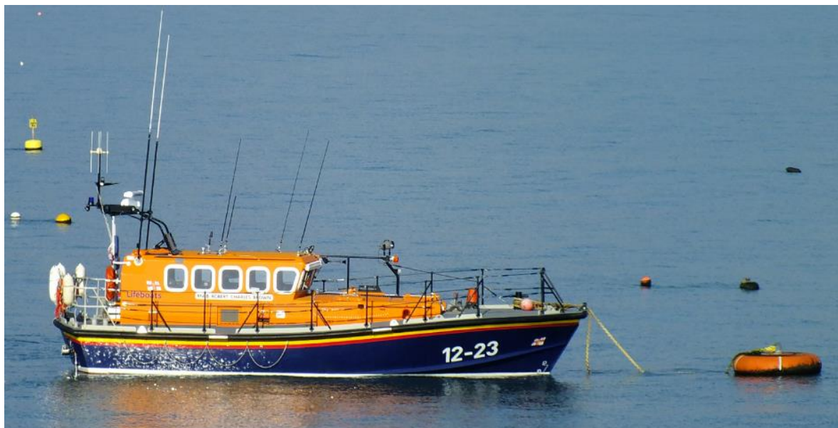
Figure 1: The Robert Charles Brown, an 11.77m Mersey class all-weather Lifeboat at a SPM.
