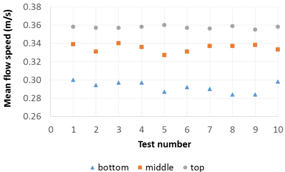
Figure 19: Mean flow measurements at three depths. Measurements are at 2Hz for 60s at depths from tank floor of 0.05m (bottom), 0.10m (middle) and 0.19m (top).
