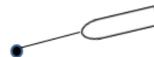
Figure 8: Fishtailing motion of a vessel at a single point mooring, adapted from Aghamohammadi and Thompson (1990).
