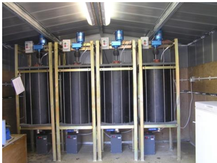
Figure 3-2 Typical schematic (left) 1 feedstock inlet; 2 motor to power a stirrer; 3 heater; 4 heating coil; and 5 digestate outlet and photo (right) of the 100-litre digesters
