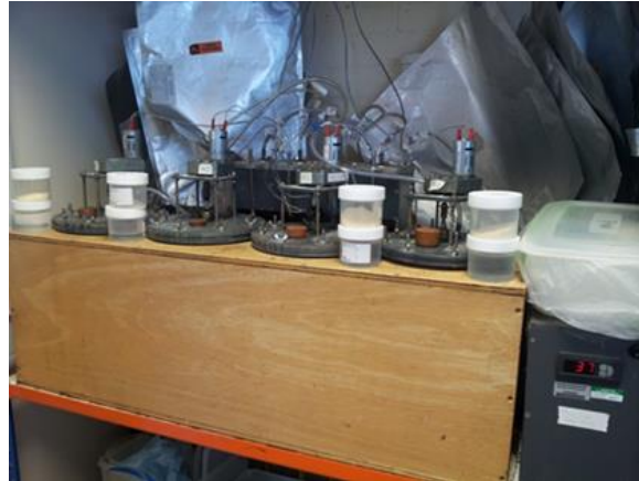
Figure 3-1 Typical schematic of the 5-litre digesters used with cross-section showing details of heating (left) and stirring systems (Banks, Zotova and Heaven, 2010; Jiang, Heaven and Banks, 2012) and photo of anaerobic digester of 5-litre digesters
