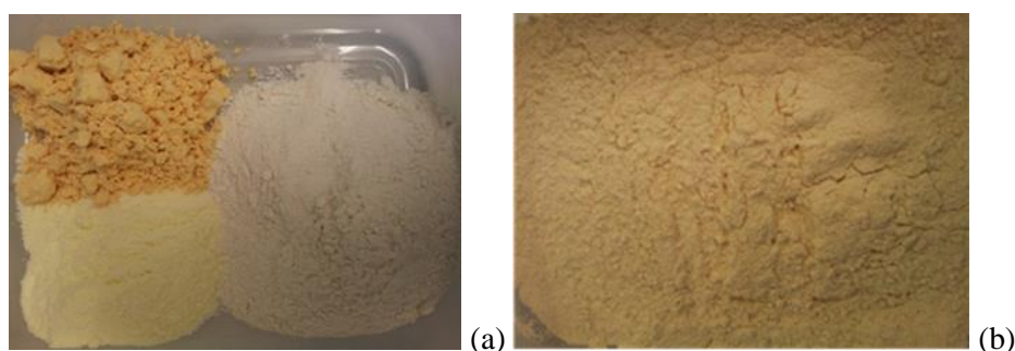
Figure 3-3 Components of the model substrate (a) top-left is egg powder, bottom-left is milk powder and right is rice flour and their mixture (b)
