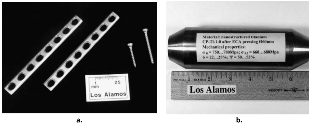
Figure 2-21 Applications of nano structured materials processed by Severe Plastic Deformation. a) implants for bone osteosynthesis made of nano structured Ti. b) Structural rod (50 mm diameter, 170 mm length) processed from ECAP billets. Adapted from [75].
