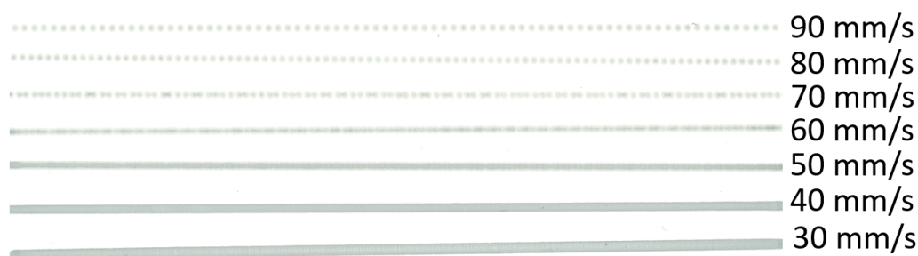
FIGURE B.1: Polymeric lines deposited on an NC membrane with different speeds in the range between 30–90 mm/s.
