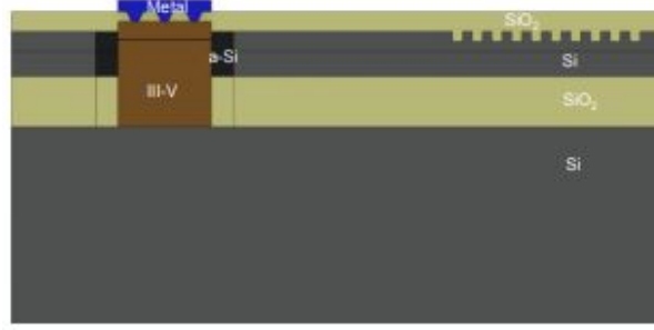
FIGURE 2.45: Cross-sectional schematic InP -based laser integrated with an SOI platform [148].
