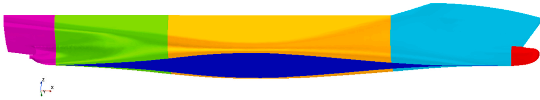
Fig. 2. KCS hull split by patch for creating heterogeneous roughness scenarios.
