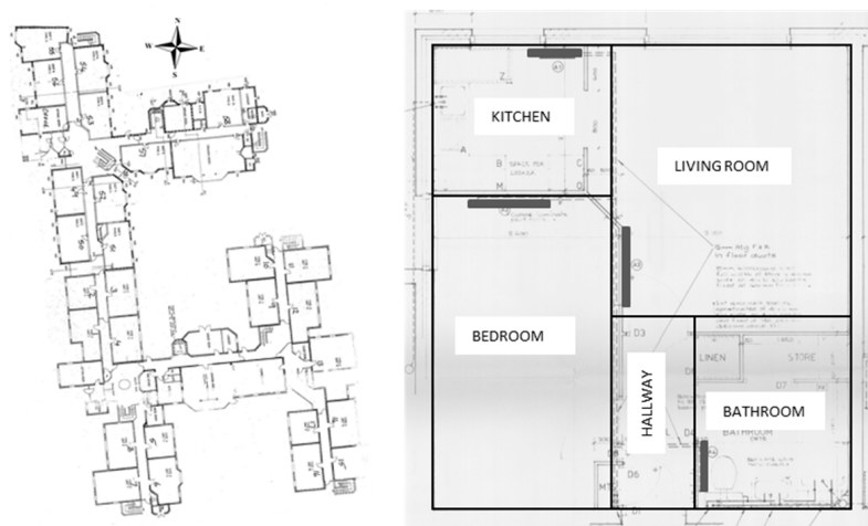
Figure 1. Building layout and typical one bedroom flat. The case study is a three-story 1984 building having 80 flats: 8 studio flats, 64 one-bedroom flats, 6 two-bedroom flats, and 2 three-bedroom flats. All flats have radiators and TRVs are the only point of control residents have of their heating.
