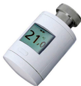
Figure 2. Smart thermostatic valves: HORA SmartDrive Mx. The smart thermostatic valves (STVs) allow users to set their desired setpoint temperature, which is displayed on the screen. The setpoint range is 10 to 30 °C. Valve aperture is regulated by the setpoint and the room temperature. Room temperature is detected by an integrated temperature sensor and corrected for temperature influences by an algorithm.
