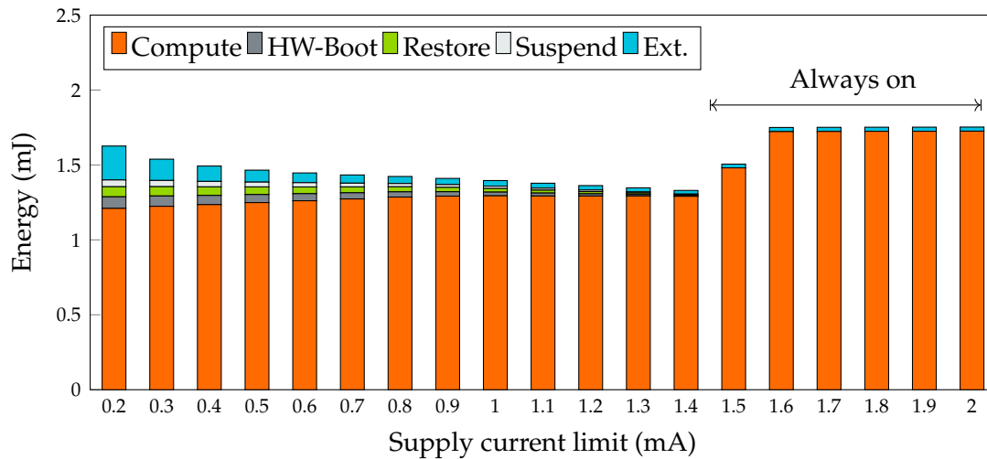
FIGURE 4.13: Full-system energy consumption when running AES encryption intermittently, powered by current-limited power source. The energy consumption is divided into stacked bars for the external circuitry ( ext. ), hardware boot ( HW-Boot ), and the operational phases restore , compute and suspend .
