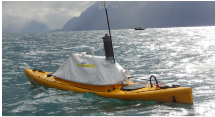
Figure 2.17: The water quality monitoring USV with an onboard pendulum energy harvester by Toh et al. (2011) .
