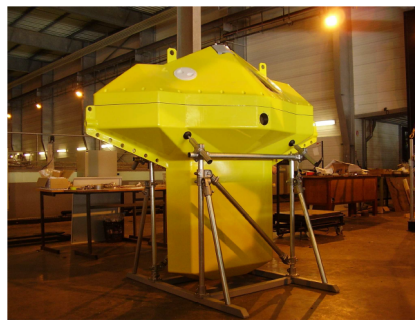
Figure 2.11: The prototype of the SEAREV G1 (Durand et al., 2007).
