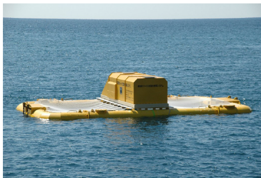
Figure 2.14: The gyroscopic moment WEC system by Kanki et al. (2009) .
