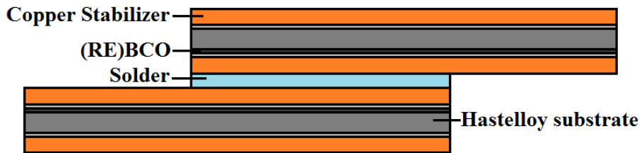
Figure 2.11: The configuration of a lap soldering joint between two 2G HTS tapes.
