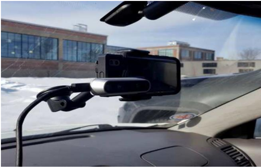
Figure 2. 4 Thermal camera and its location for data capture (Nowruzi et al. 2019)
