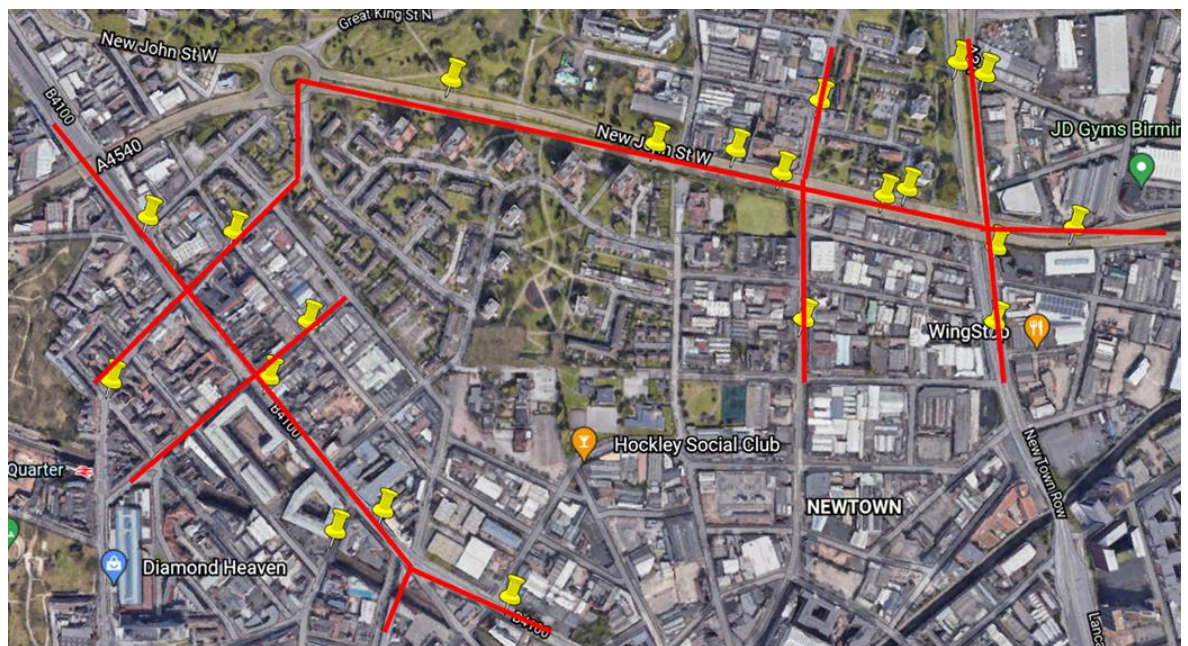
Figure 5. 1 Map of the case study location in the Newtown area of Birmingham. The locations of inductive loops are marked with yellow probes. The lane approaches are represented by red lines
