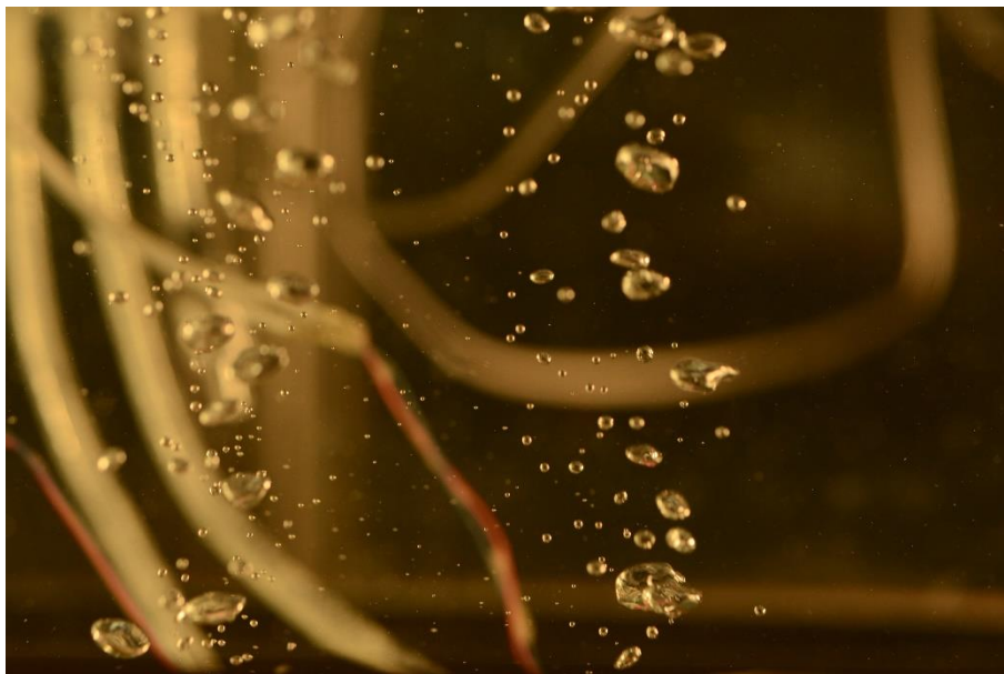
Fig. AC 2: Example of frame for air flow equivalent to 10 \text{ L min}^{-1} ( 5 \text{ L min}^{-1} \text{ m}^{-1} ) at 2 bar, vibration 2.2V.
