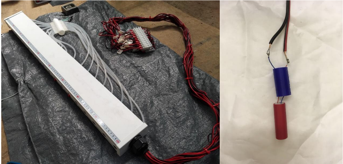
Fig. 4.2 – Left: External view of one of the two bubblers used for this study. For health and safety reasons, injection needles were fitted into place once bubbler was positioned inside the flume. Right: Close-up of the 3D-printed cylindrical housing and vibrating motor.
