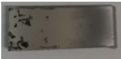
Figure 4-17: Image of a tile containing GeTe. (Note: the scratch marks occurred during the electrical and thermoelectrical measurements).
