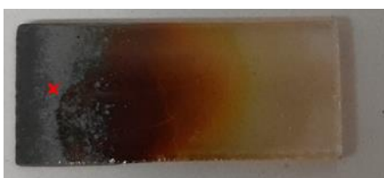
Figure 4-12: Image of a tile containing highly orientated GeSe. The red cross indicates the region investigated for characterisation.
