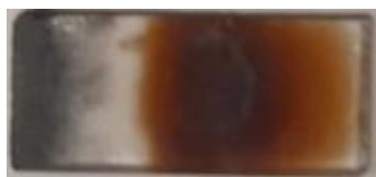
Figure 4-7: Image of the small amount of deposited GeS (grey material at left hand side of tile).
