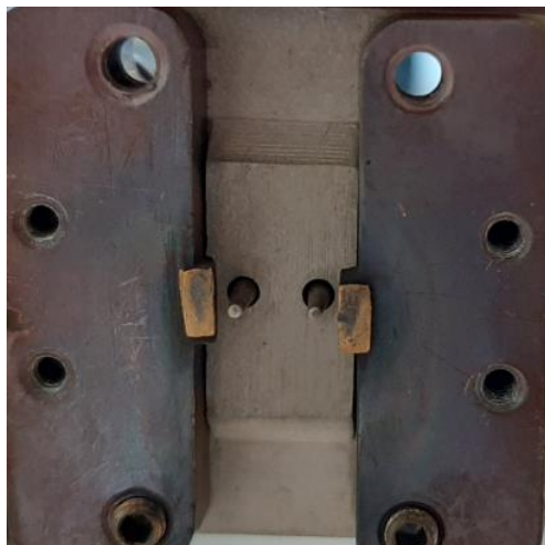
Figure 1-24- The probe set up for the variable temperature Seebeck coefficient and resistivity measurement equipment. The outer probes control the temperature gradient across the film and the two central smaller probes measure voltage for the resistivity measurement.
