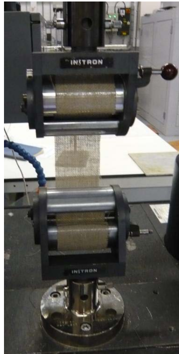
Figure 11: Tensile test of a cloth specimen
