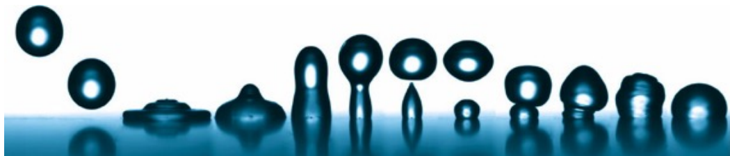
Figure 11 Reprinted from [49], illustration of a rebounding droplet impact
