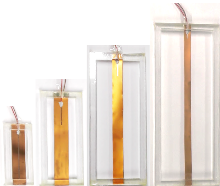
Figure 112 Photograph of AF = 35 mm spiral equivalent length fixed-fixed beams. Beams represent spiral arm width and length in a straight, fixed-fixed beam format. From left to right, fixed-fixed beam equivalent of a 0.25, 0.5, 0.75 and 1 turn samples
