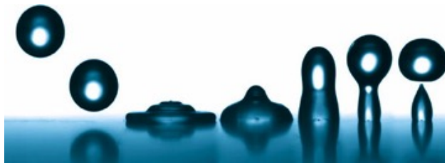
Figure 105 Reprinted from [49], image illustrating droplet spreading on impact
