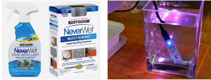
Figure 10 Left image, reprinted from [46], example of hydrophobic spray product “NeverWet”. Right image, reprinted from [47], depicts an Arduino Micro Board circuit in water. This circuit was coated by super-hydrophobic coating “NeverWet” [46], and continued to operate in a submerged environment
