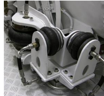
Figure 6. 9 Vibration control system
