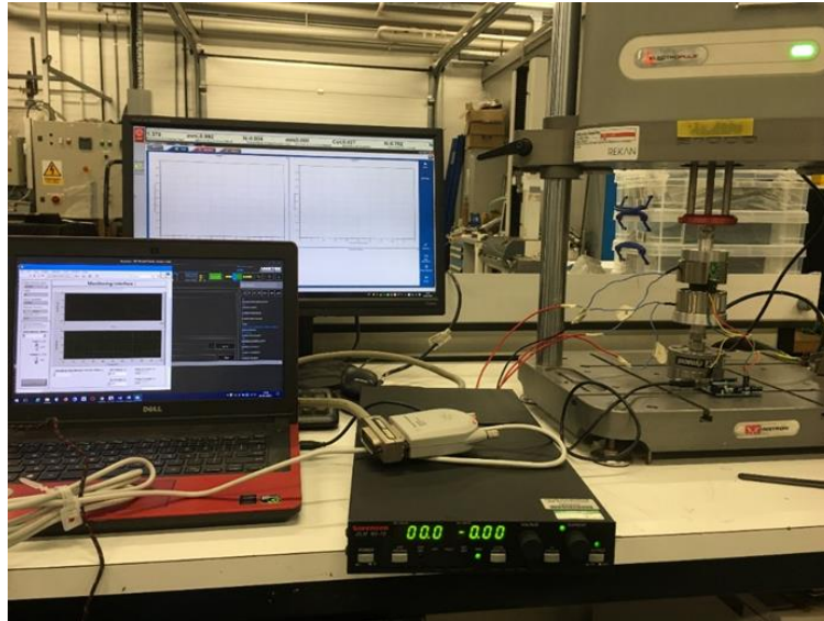
Figure 6.23 Experiment setup of the semi-active MRE mount test.
