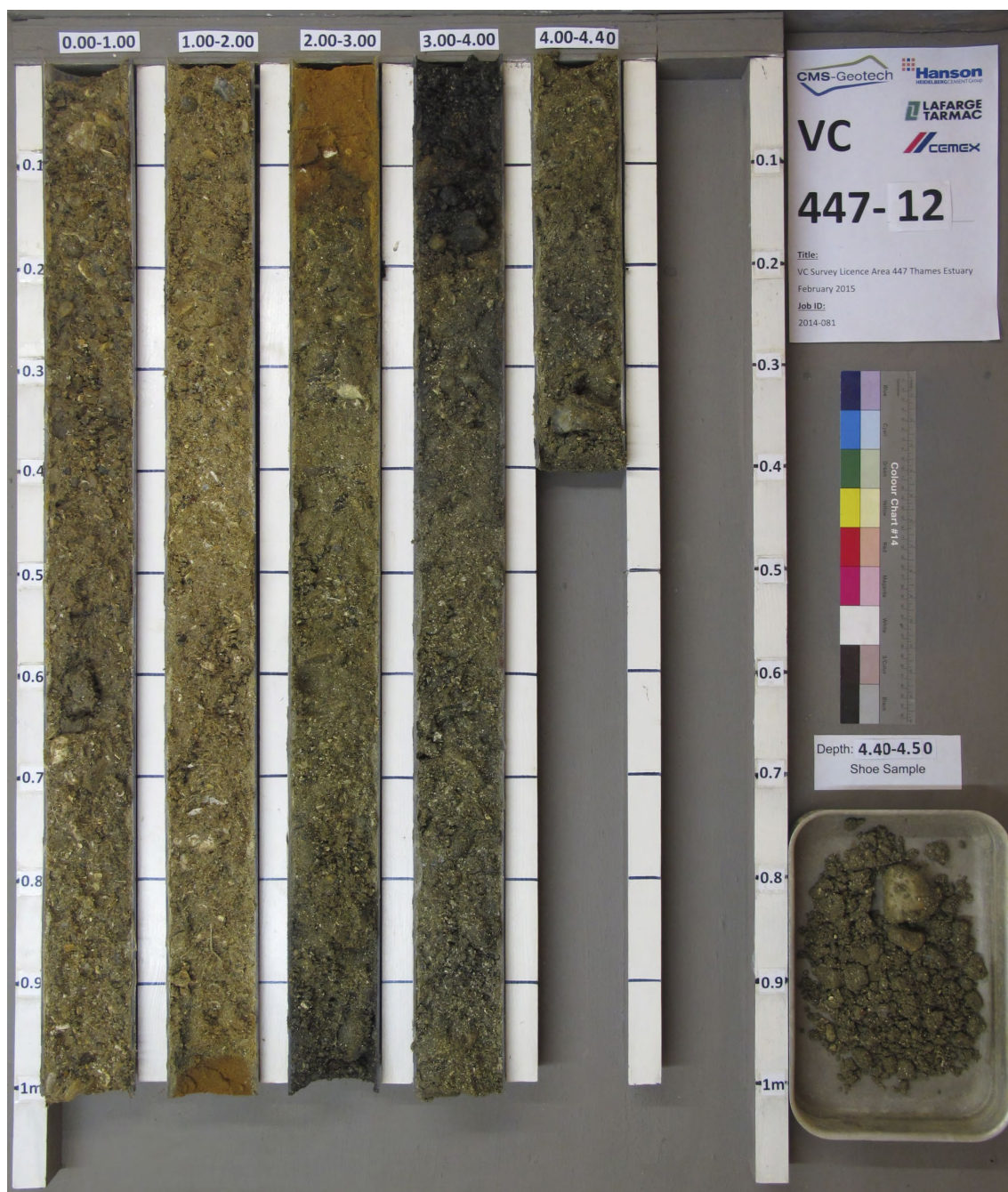
Figure 21 Photograph of vibrocore VC12
