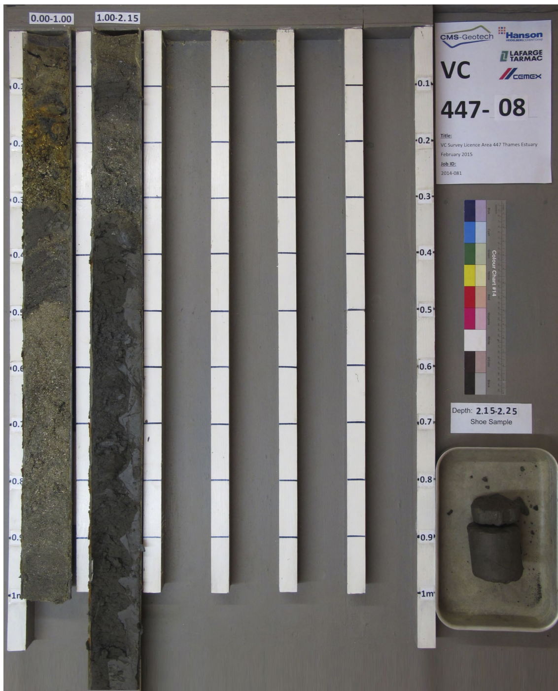
Figure 19 Photograph of vibrocore VC08
