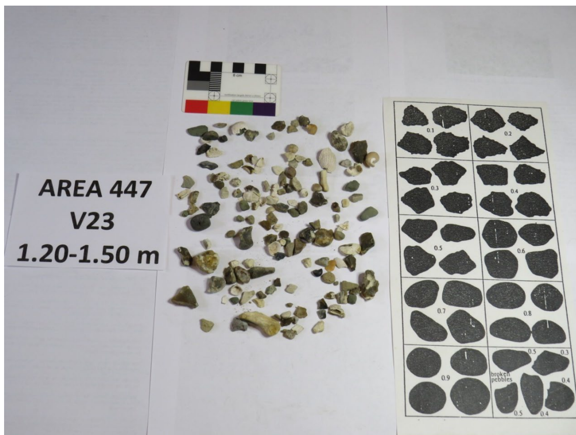
Figure 26 Lithological sample 1.20–1.50 m retained after sieving
