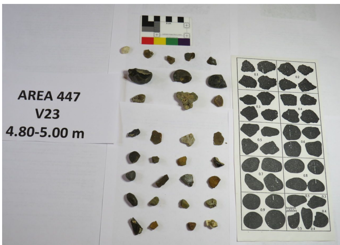
Figure 28 Lithological sample 4.80–5.00 m retained after sieving
