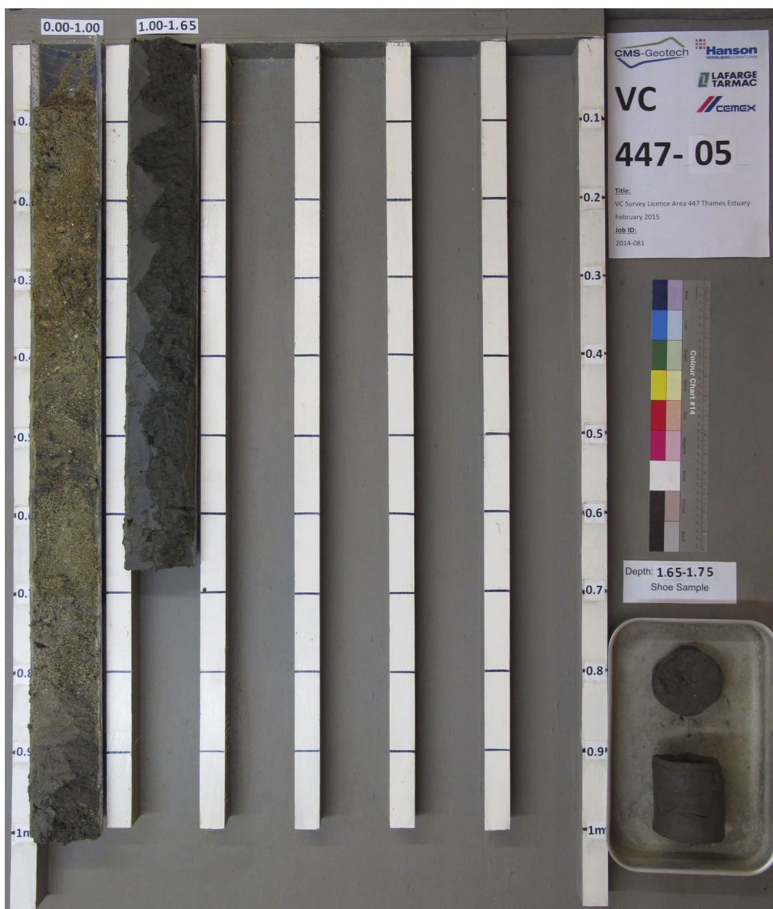
Figure 18 Photograph of vibrocore VC05
