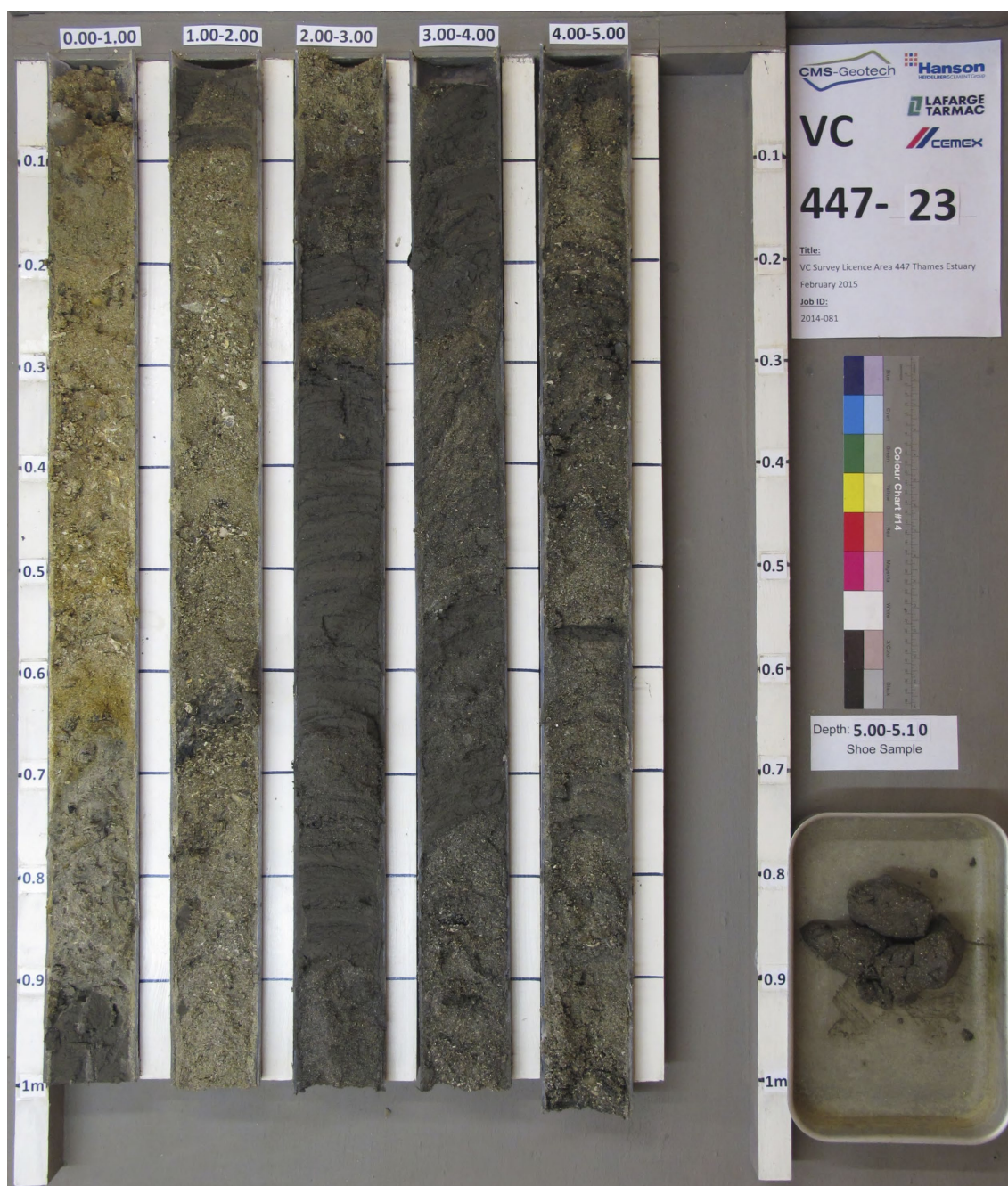
Figure 24 Photograph of vibrocore VC23
