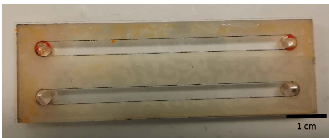
Figure 33 Example of a flow cell subjected to leakage testing, which failed upon exposure to a flow rate of 25 mL/min. There is indication of leakage of fluid and precipitation of the dye into the tape bonding the glass surface to the acrylic manifold.
