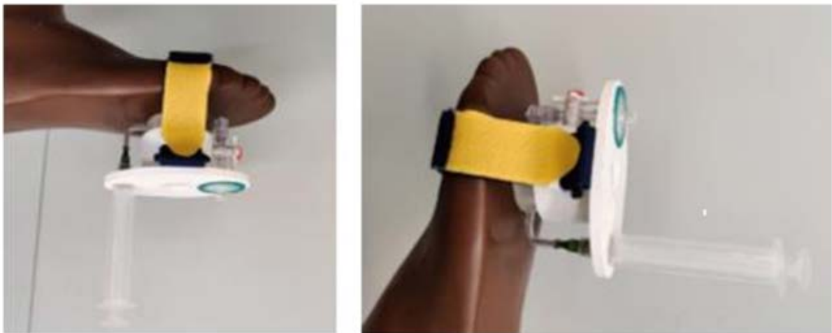
Figure 90 The device is shown attached to the model foot whilst pronated (facing downwards) and supinated (facing upwards) to demonstrate the versatility of the device. All components remained securely positioned within the cover piece, and no leakage from the coupon was seen. The coupon in these experiments was filled with water, to prevent damage or staining of the loaned prosthetic foot.
