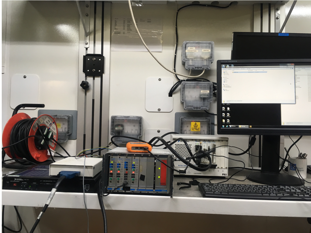
FIGURE 4.3: Hardware to induce and measure roll motion on scale vessel in towing tank
